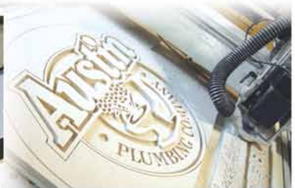
Triad CNC carves dimensional signs out of high-density urethane
